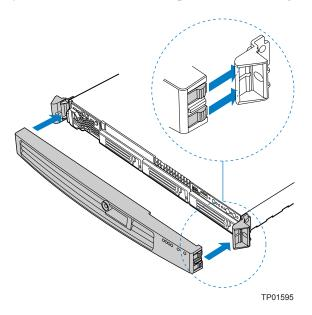
Figure 12. Installing the Front Bezel
